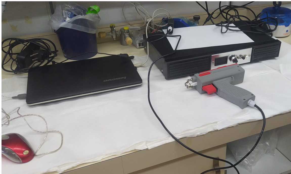
The e-Biopsy research system, including the High-Voltage Pulse Generator (BHVP) and the specialized aspiration handheld probe
